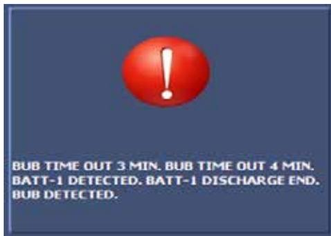
When cart is connected it shows the State of Charge of Battery 1 (BATT-1) and Backup Battery (BUB)
